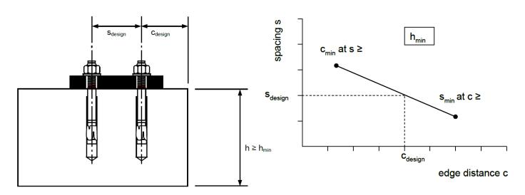
FIGURE 2 – INTERPOLATION OF MINIMUM EDGE AND SPACING DISTANCE
