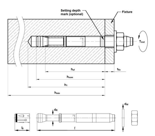
FIGURE 1 - HILTI HST3 AND HST3-R INSTALLATION PARAMETERS AND GEOMETRY
