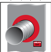
5. Fasten identification plate (if required)
